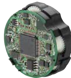
Figure 1 Exterior of Mechanical Absolute Encoder
